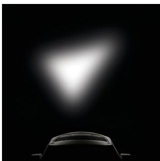
Individually controllable blades with variable angle (+/-28°) and position
